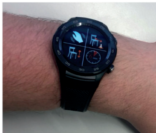
Figure 2. The Huawei Watch 2 worn on the left wrist, showing the interface. The interface shows four icons, one icon for each of the four tests. 1) 4SBT (upper left icon), 2) TUG (upper right icon), 3) 30STS (lower left icon), 4) 6MWT (lower right icon).
