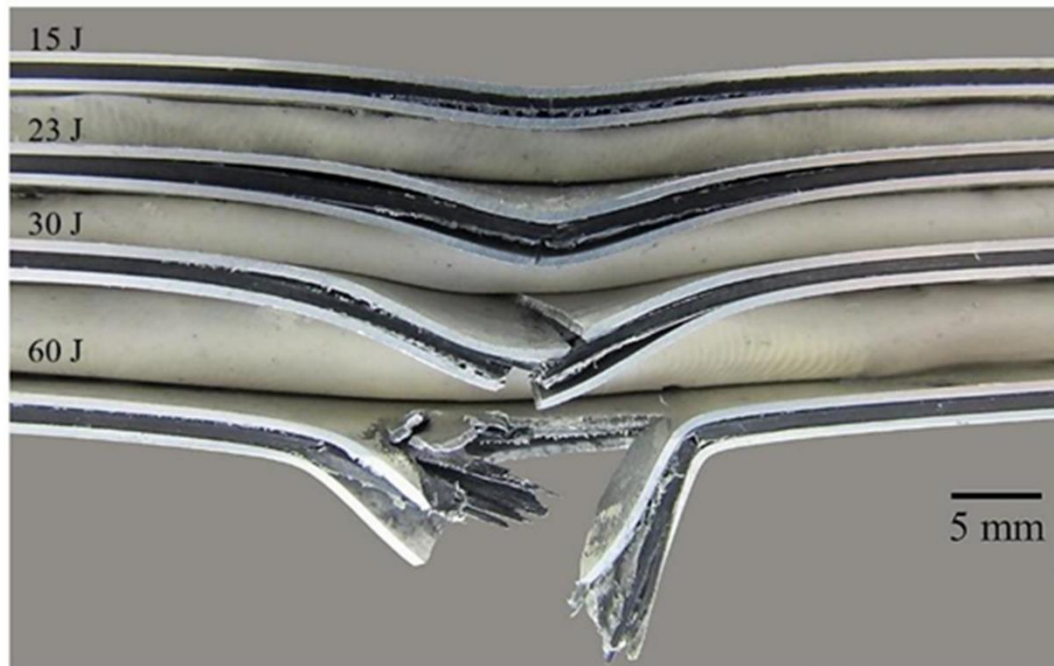
Figure 11. Cross sections of FML 2/1 at different impact energies.
