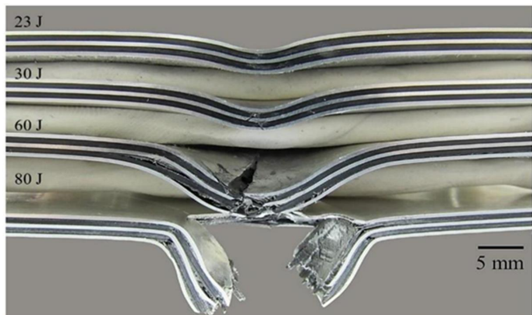
Figure 12. Cross sections of FML 3/2 at different impact energies.
