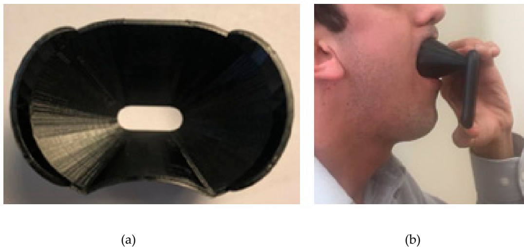
Figure 2. Our developed add-on gadget and its usage for data acquisition. (a) Add-on gadget designed and manufactured by 3D printing, and (b) image acquisition setup using the iPhone X with the add-on gadget.
