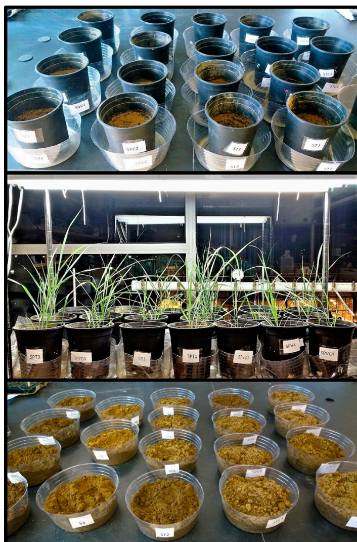
Figure 1. (Top): Pots containing contaminated soils amended with the different organic treatments without switchgrass placed over plastic containers used for leachate collection, (Middle): Vegetated pots containing switchgrass growing in laboratory under 24-h light conditions, (Bottom): Soil that was removed from the pots at the end of the experiment for analysis.
