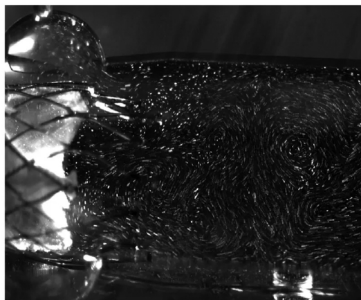
VIDEO 8. Raw video showing the flow downstream of the Allegra (New Valve Technologies). Video available at: https://www.jtcvs.org/article/S2666-2736(22)00168-1/fulltext .
