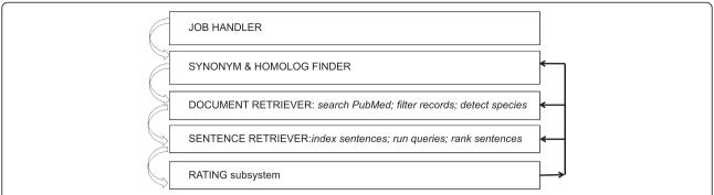
**Fig. 1** System components. The figure shows processing sequence with the arrows on the left side. The user may modify aspects of the job (homologs, synonyms etc.) at several points as shown by arrows on the right
