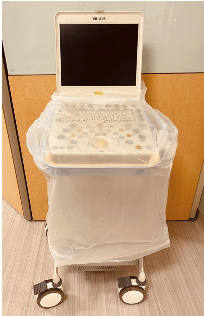
Fig 2. Compact ultrasound machine prepared for coronavirus disease–2019 veno-venous extracorporeal membrane oxygenator cannulation. All extraneous cords removed with a single-phased array probe connected.
