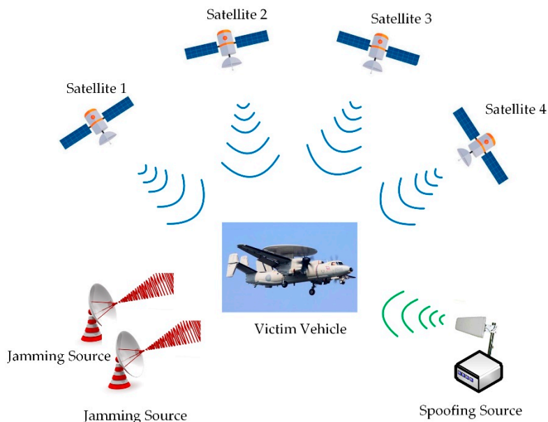
Figure 1. Illustration of an intentional attack on a global navigation satellite system (GNSS) receiver mounted on an aerial vehicle.
