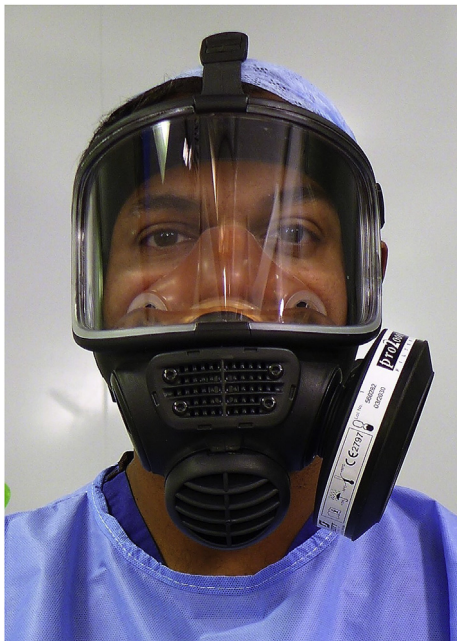
Fig. 2. Full-face air-purifying respirator (APR).
