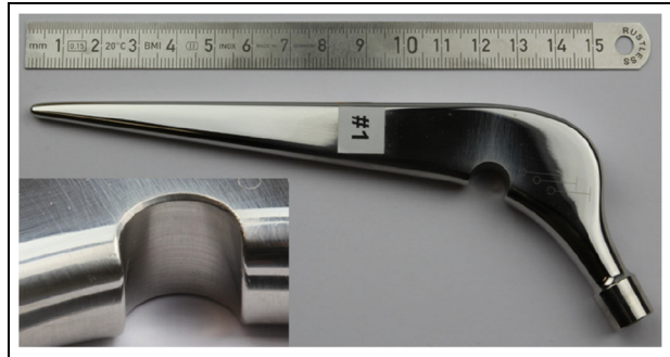
Figure 2. Modified implant geometry with detail of the milled cavity. The new surface showed a rougher structure from milling and polishing than the original mirror finish.
