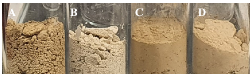
Figure 2. \text{FeCO}_3 product synthesized at 24 h and 130 °C. The synthesis has been carried out as a function of pressure. (A) 1, (B) 5, C) 10 bar (different batch compared to Figure 1), and (D) 15 bar.
