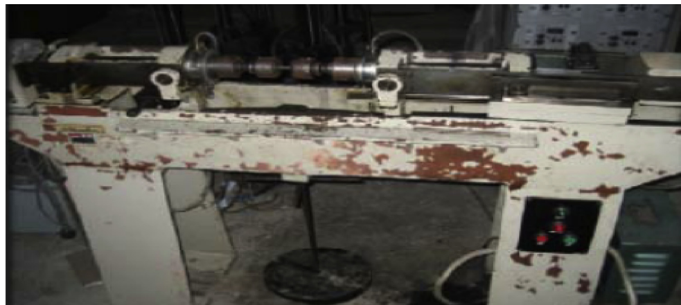
Figure 5. Rotary bending fatigue test.
