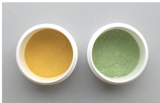
Figure 11. ITO powder sample, before (left) and after (right) TPD in He, showing a discoloration from yellow to greenish-gray.
