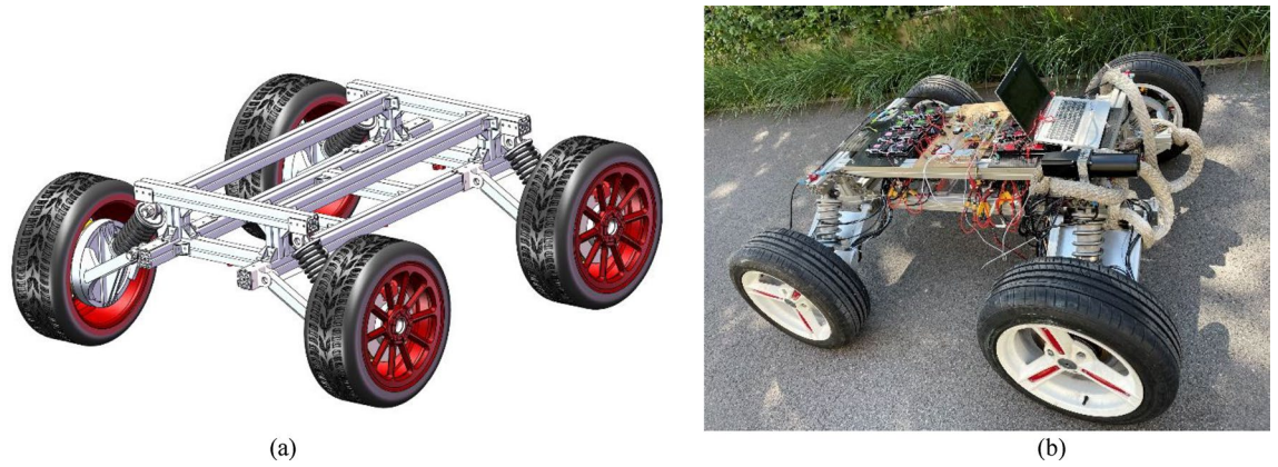
Figure 2. (a) A designing diagram using SolidWorks, (b) actual UGV used in this work.
