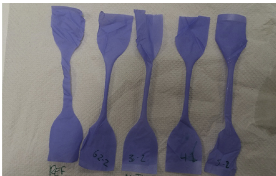
Figure 2. Test specimens obtained (UNE-EN ISO 527-3 Type 5).
