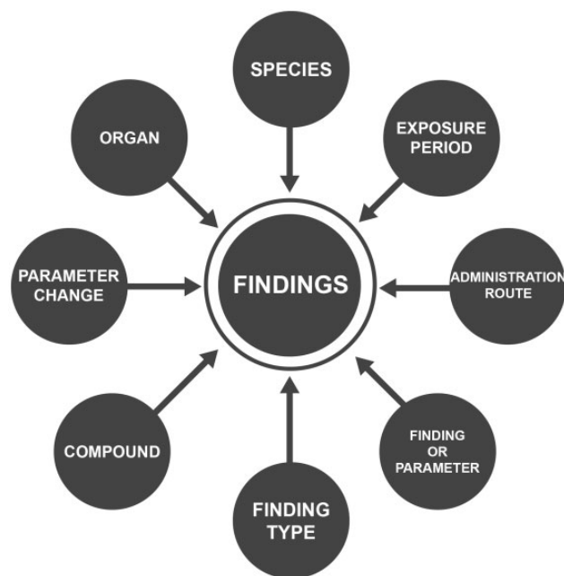
Figure 3. OLAP schema. Schema of the multidimensional data model used to build the data extraction mechanism. Findings are modeled as facts in a multi-dimensional space, located at the center and connected to the dimensions around, describing 8 different properties: species, organ, parameter change, compound, finding type, finding/parameter, administration route and exposure period.
