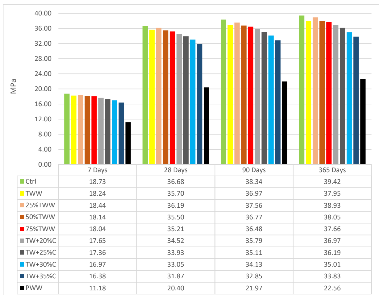
Figure 3. Compressive strength cured by drinkable water.
