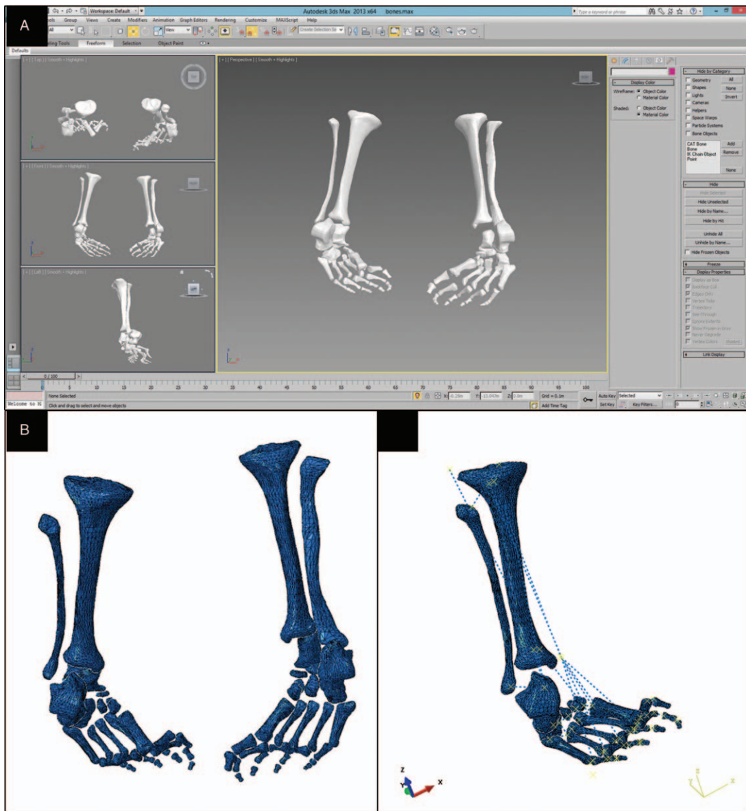
Figure 2. Steps for computational simulation. (A) Importing of 3D elements in *.sat format; (B) assembling of solid elements; (C and D) introducing of connectors and tendon-type elements in the system.
