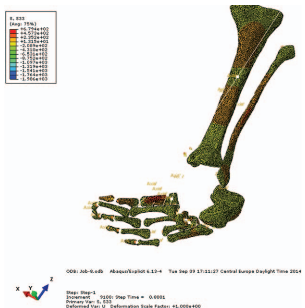
Figure 7. Von Mises equivalent stress distribution in the simulated foot.
