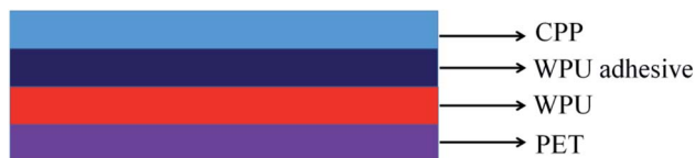
Fig. 2 Schematic diagram of PET/CPP laminate film samples for the measurements of T-peel.
