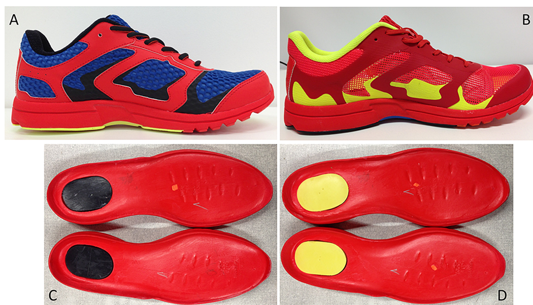
Figure 1 Image of shoes prototypes used in the experiment. Illustration of testing shoes. (A) Structured Upper condition (SU). (B) Minimalist Upper condition (MU). (C) Low Resilience cushioning material condition (LR). (D) High Resilience cushioning material condition (HR).
