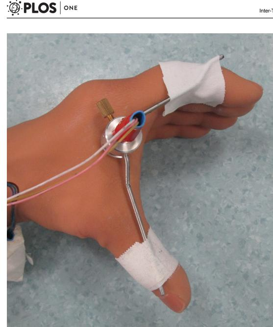
Fig 3. Potentiometer attached to the prosthesis hand.
