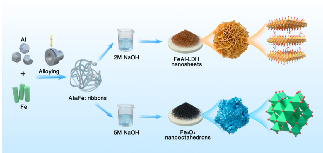
Figure 1. Schematic illustration showing the corrosion-engineered fabrication process of the FeAl-LDH nanosheets and \text{Fe}_3\text{O}_4 nanooctahedrons.
