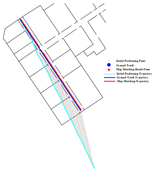
Figure 32. Positioning results of the geometric algorithm on Route 1 (Narrow corridor).
