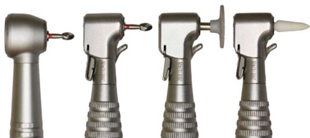
Figure 1. High-speed tungsten carbide bur (BurH; BurH-cool); low-speed tungsten carbide bur (BurL); low-speed aluminum-oxide disc (DiscL); and low-speed fiberglass bur (BurFGL)
