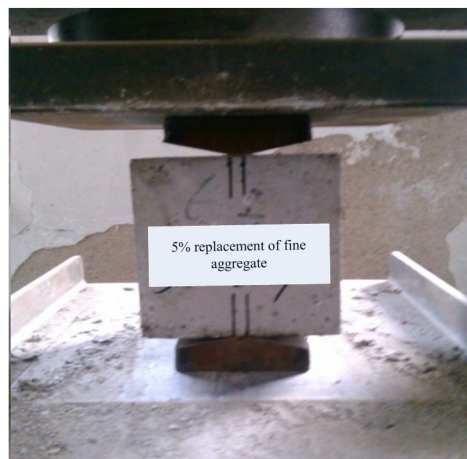
Figure 4. Splitting tensile strength test.
