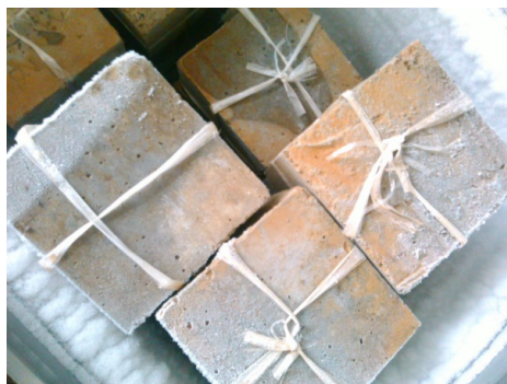
Figure 6. Freezing-thawing of crumb rubber concrete.
