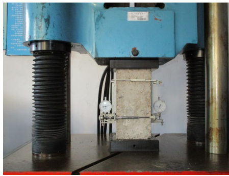
Figure 5. Modulus of elasticity test.
