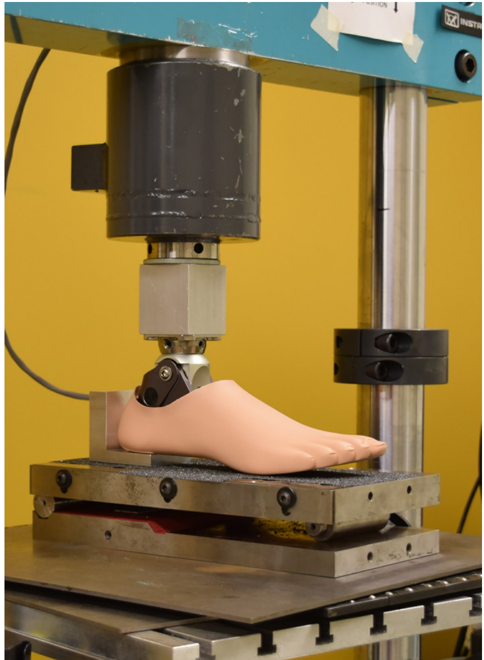
Fig 3. Test set up for the barefoot midstance condition, including the heel (L-)block.
