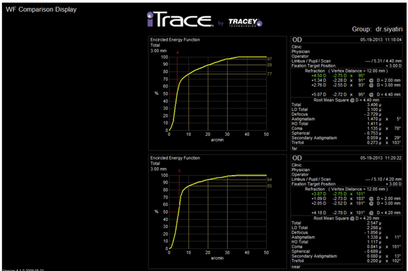
Fig. 2. The point spread function (PSF) is used to calculate the encircled energy function (EEF).
