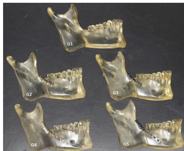
Fig. 1: Photoelastic models. Non-fractured control hemimandible (G1) and fractured hemimandibles fixed by different osteosynthesis methods (G2: four-screw conventional plate, G3: four-screw locking plate, G4: seven-screw conventional plate, and G5: seven-screw locking plate).
