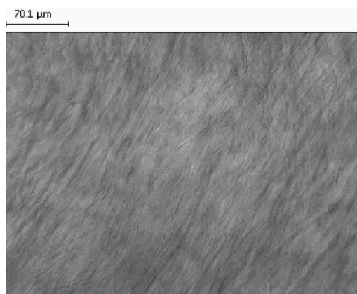
Figure 1. Polarizing microscopic examination of blank lyotropic liquid crystal systems (LLC) at a magnification of 20×.
