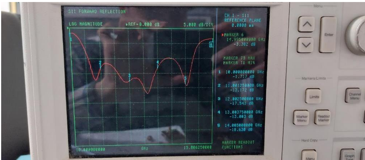
Figure 4. Simulated and measured S_{11} and the realized gain of the fabricated patch array.
