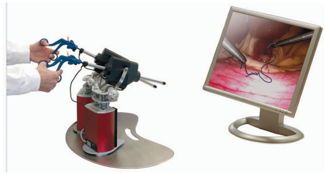
Figure 1 VR simulator example. Hardware: Xitact® (Xitact S.A., 1110 Morges, Switzerland), software: LapSim® basic tasks module (Surgical Science, SE 413 14 Göteborg, Sweden)
