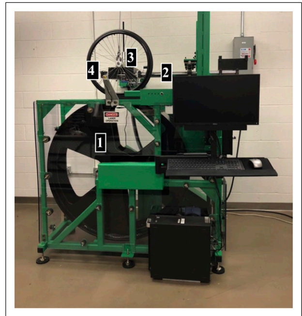
Figure 1. Component-level test equipment 1) rotating drum 2) arm assembly 3) air bearings 4) primary load cell.
