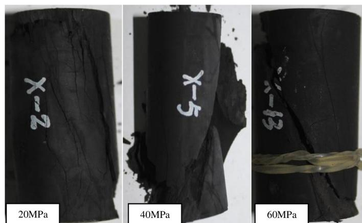
**Fig 8. Fractured samples after unloading with different initial confining pressures.**
