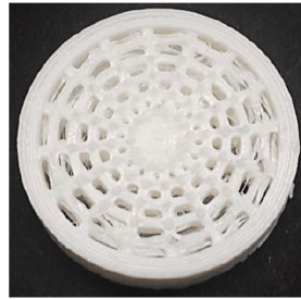
Figure 1. The 3D printer stringing effect appearance of a preliminary sample.
