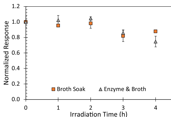
Figure 4. Leached lactic acid from PLLA samples in M4 broth as quantified with LC versus UV light degradation time and normalized to the values of the 0 h (pristine) sample. Markers represent the average ( n = 3 ) with the error bars representing the standard deviation. “Broth Soak” are plastic samples that are similar to those in the nonenzymatically treated polymer sample whereas “Enzyme and Broth” are the samples in the enzymatically pretreated sets.
