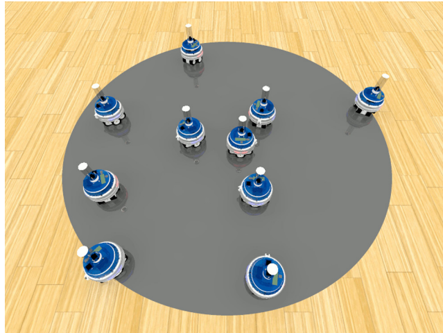
Fig 5. Setup of the flocking experiment. Ten robots are initialised randomly within a circle of 1 m radius (see grey circle) with random orientation. Each robot displays a coloured left-right pattern with red and blue LEDs to provide information about its heading direction (see S1 Text for more details). Experiments are performed in simulation [21].
