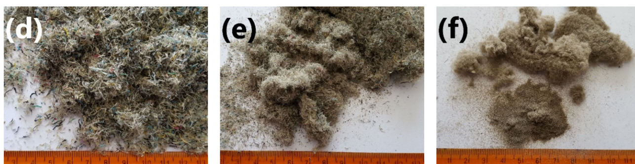
Figure 2. The appearance of M1, M2, M3 wastes and impurities removed during washing and retained on sieves with (a) 4 mm, (b) 2 mm, (c) 1 mm, (d) 0.5 mm, (e) 0.125 mm, and (f) residue.
