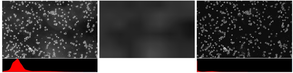
Fig 4. Illumination correction: Original image (left), estimated noise (middle) and the corrected image (right).
