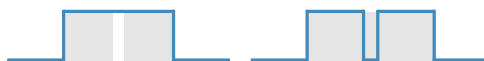
Fig. 8 False annotations that are very mildly punished when evaluating per timestamp using F_1 -score or similar. The blue line represents the real event segment, the gray area shows the predicted event segment. On the left the real event segment is predicted as two segments, and on the right two real event segments are predicted as a single one. In both cases the Jaccard-Time-Span-Event-Score (JTES) will result in a score \leq 0.5 .
