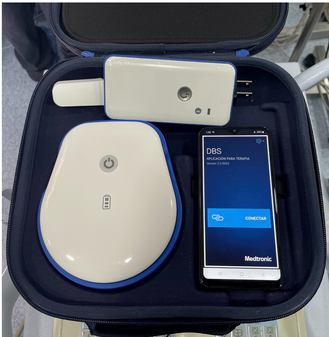
Fig. 1. Wireless patient programmer for the DBS. This device allows changing parameters and turning the DBS on and off.
