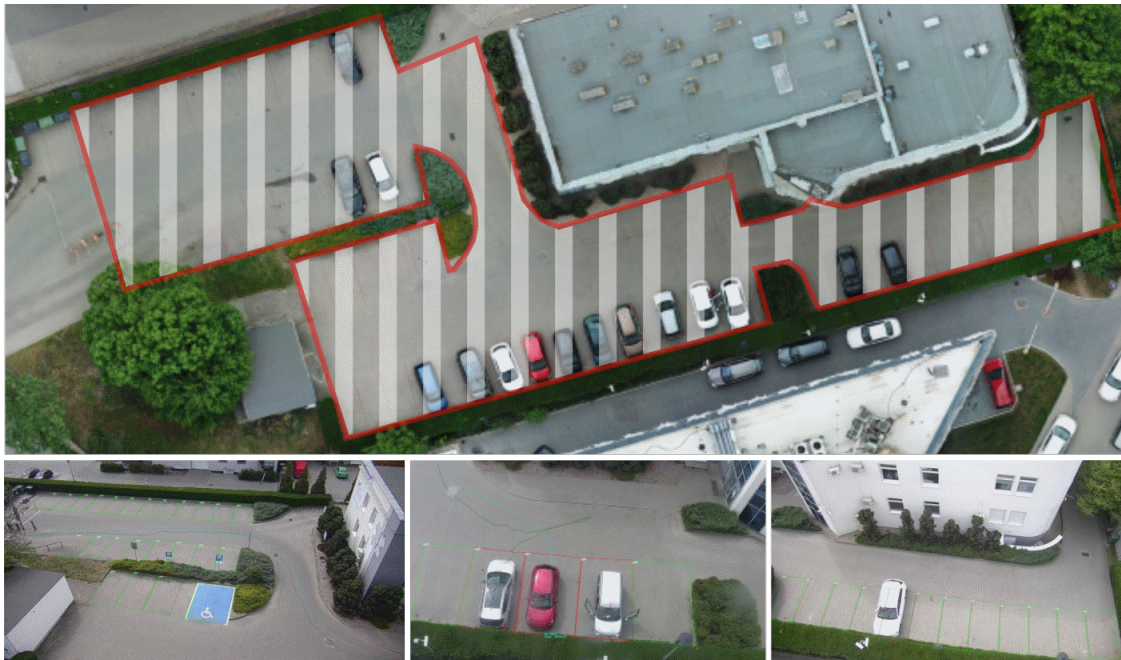
Figure 8. Simple multi-camera tracking system for a parking. The cameras track the vehicles from the barrier to the parking space.
