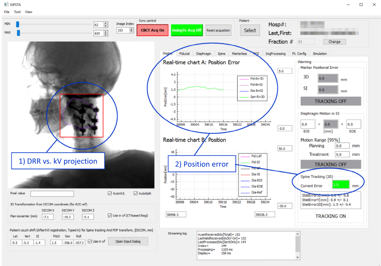
Figure 1 Graphical user interface of KIPSTA. For spine tracking, KIPSTA displays the following: 1) comparison between DRR and kV projection, and 2) position error (color-coded green box turns red when the detected error is larger than a threshold). Of note, KIPSTA was developed for multiple tracking modes including fiducial marker and diaphragm tracking although only data relevant to spine tracking is displayed.
