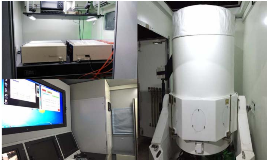
Figure 3. Physical map of our ground-based CO 2 -DIAL system.
