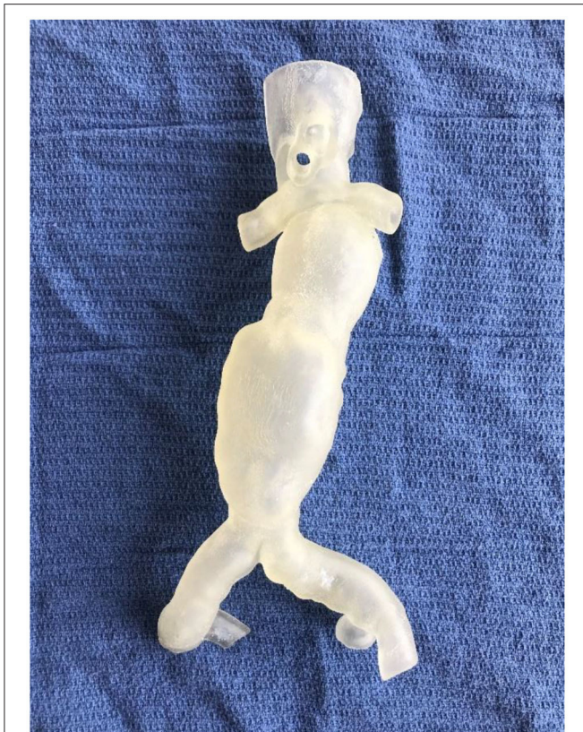
FIGURE 8 | A flexible, hollow, translucent AAA phantom 3D printed using Inkjet technology.
