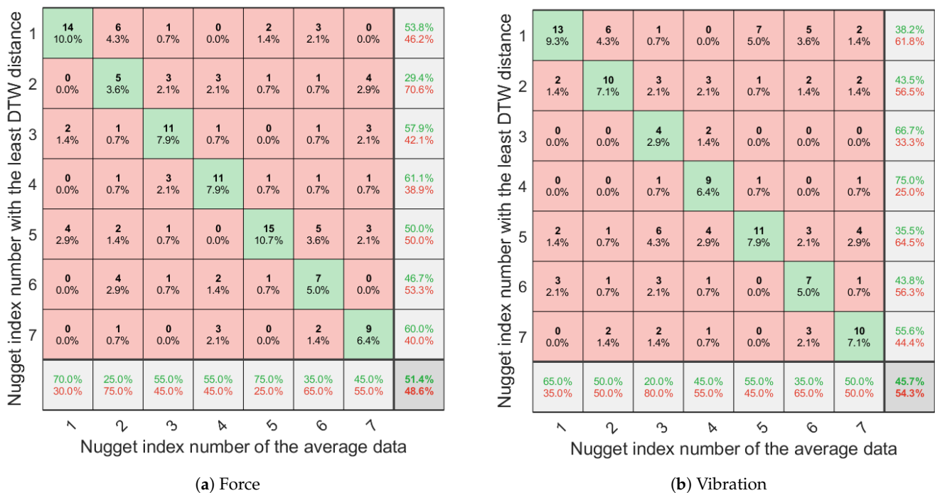
Figure 10. Confusion matrixes of force and vibration. The numbers and percentages were calculated for when the DTW distance in the average data for nuggets with the same coating was least compared to the DTW distances for the average data of other nuggets with different coatings. The green number indicates the percentage which the nugget index number with the least DTW distance and the nugget index number of the average data matched. The red numbers indicate the percentages that did not match.
