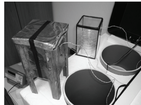
FIGURE 4: Control samples (left, shielded) and exposed samples (right, unshielded) holders.
