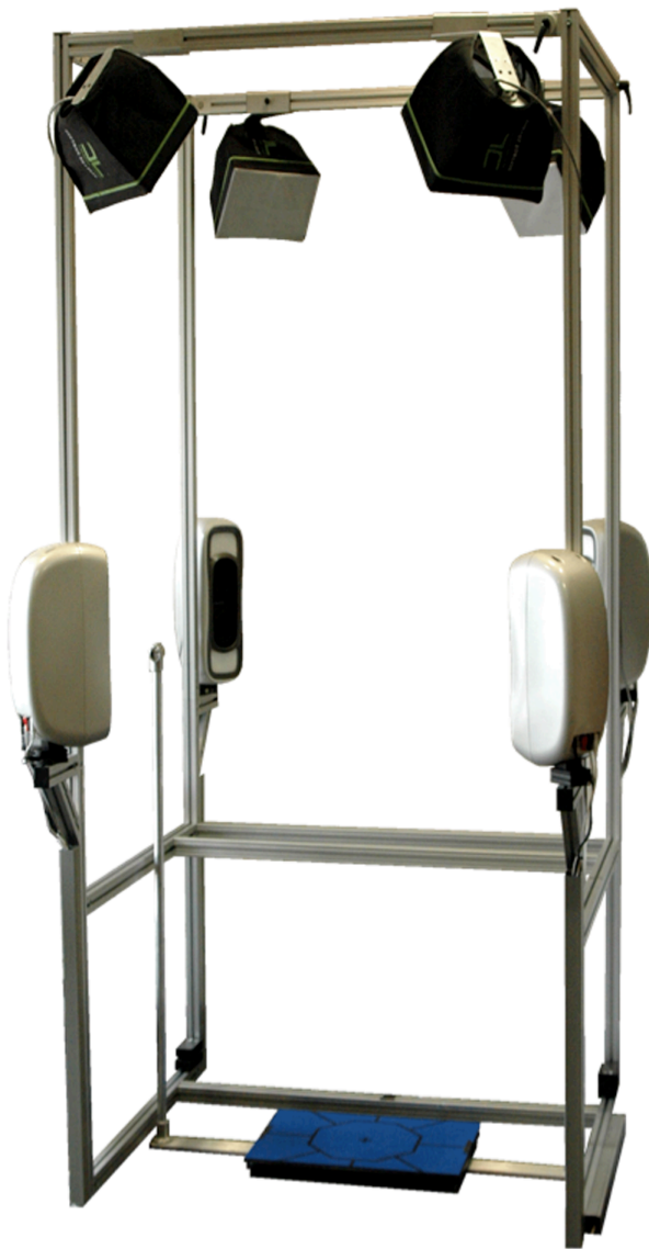
Figure 3. The Vectra 3D scientific photographic station.
