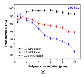
**Figure 10.** The influence of the kaolin concentration on the samples transmittance: AMD/ALg II obtained at 0.5 kGy (**a**), 0.75 kGy (**b**), 1 kGy (**c**), 1.25 kGy (**d**), 1.5 kGy (**e**), 1.75 kGy (**f**), and 2 kGy (**g**).
