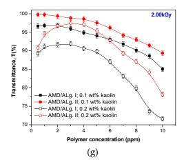
**Figure 9.** The influence of the polymer type and kaolin concentration on the samples transmittance: AMD/ALg I and II obtained at 0.5 kGy (a), 0.75 kGy (b), 1 kGy (c), 1.25 kGy (d), 1.5 kGy (e), 1.75 kGy (f), and 2 kGy (g).
