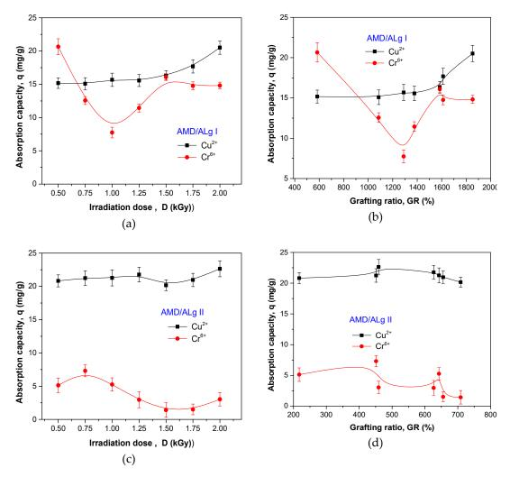
**Figure 12.** The influence of irradiation dose, grafting ratio, and sodium alginate concentration on equilibrium absorption capacity. (a) absorption capacity versus irradiation dose for AMD/ALg I samples; (b) absorption capacity versus grafting ratio for AMD/ALg I samples; (c) absorption capacity versus irradiation dose for AMD/ALg II samples; (d) absorption capacity versus grafting ratio for AMD/ALg II samples.
