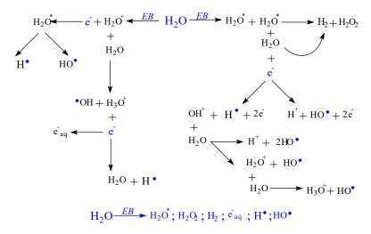
Figure 4. Possible mechanism for obtaining radicals by irradiation from water.
