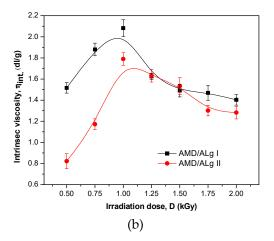
**Figure 1.** Conversion coefficient (**a**) and intrinsic viscosity (**b**) versus electron beam irradiation dose for AMD/ALg I and AMD/ALg II polymer types.
