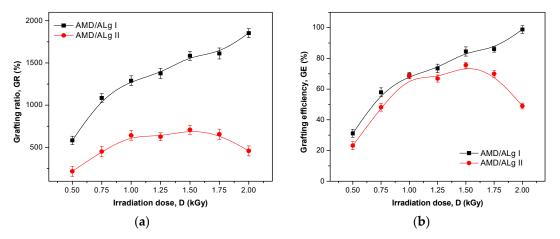
**Figure 2.** Grafting ratio (**a**) and grafting efficiency (**b**) as a function of sodium alginate concentration and irradiation dose.
