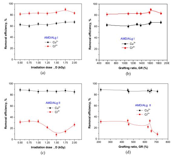
**Figure 11.** The influence of irradiation dose, grafting ratio, and sodium alginate concentration on  $Cu^{2+}$  and  $Cr^{6+}$  ion removal efficiency. (a) removal efficiency versus irradiation dose for AMD/ALg I samples; (b) removal efficiency versus grafting ratio for AMD/ALg I samples; (c) removal efficiency versus irradiation dose for AMD/ALg II samples; (d) removal efficiency versus grafting ratio for AMD/ALg II samples.
