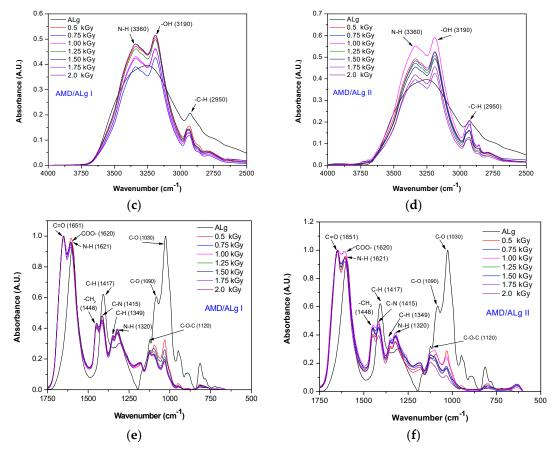
**Figure 3.** The FTIR spectra of AMD/ALg I (a) and AMD/ALg II (b) samples. Details of the AMD/ALg I (c), AMD/ALg II (d) spectra between 4000–2500 cm $^{-1}$  and AMD/ALg I (e), AMD/ALg II (f) spectra between 1750–500 cm $^{-1}$ .
