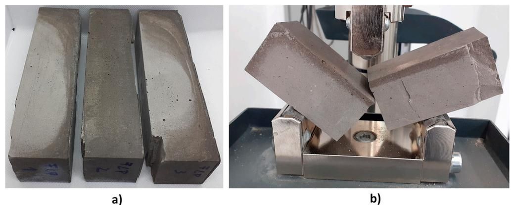
**Figure 4.** Samples made of mixture FBC FA + M (25%) demolded after 7 days; picture taken after 28 days of curing (a) before the strength tests; (b) during the three-point bending test.
