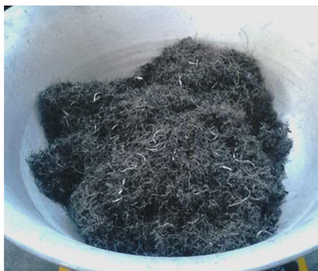
Figure 2. Recycled steel fibers used in the investigation.
